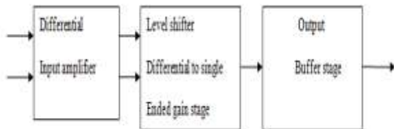
Figure1: The general structure of operational amplifier
