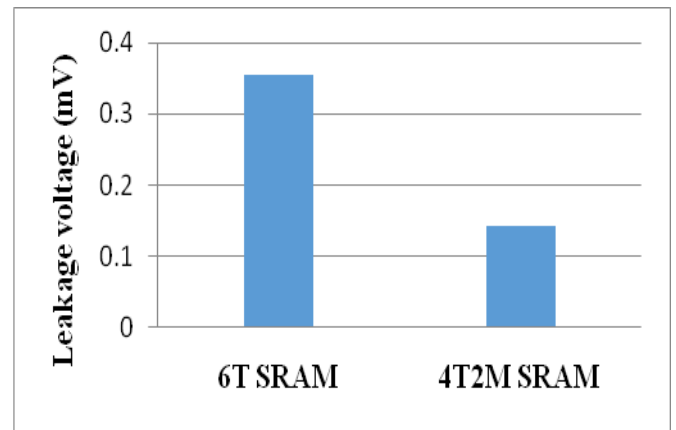
Figure 17. Comparison of leakage voltage of both cells.
