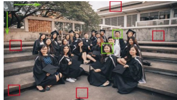
Figure 4: Detection of Sliding-Windows Detection process through Viola-Jones.
