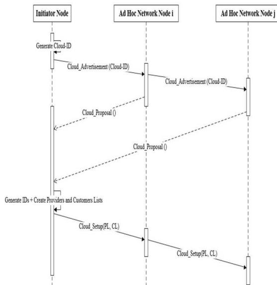
Figure 2. Sequence Diagram of the Setup Phase
