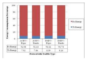
**Figure 5:** Energy consumption percentage of total transmission and receiving energy with 30 nodes
