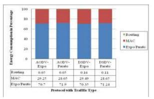
**Figure 1:** Energy consumption percentage due to packet type during transmission and reception with 10 node
