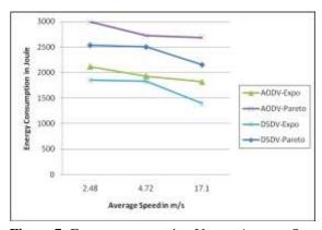
**Figure 7:** Energy consumption Versus Average Speed with 50 nodes
