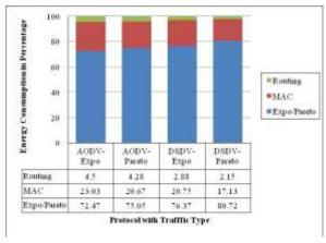
**Figure 3:** Energy consumption percentage due to packet type during transmission and reception with 50 nodes
