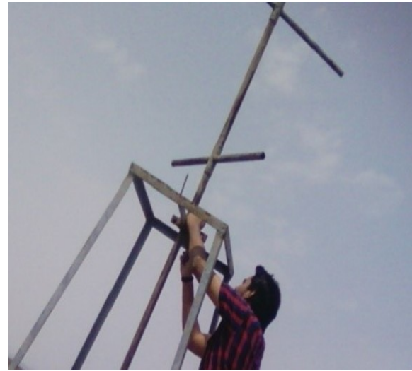
Figure 8: Fitting Central Shaft on Upper Bearing
