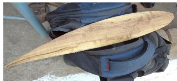
Figure 9: Wooden Block Piece in Shape of Required Aerofoil
