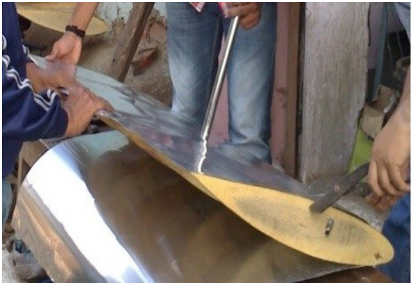
Figure 11: Wrapping Aluminum over Skeleton of Blade
