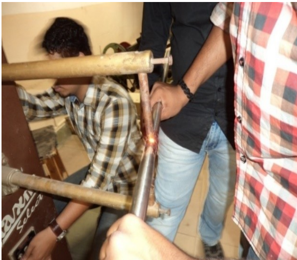
Figure 7: Welding Central Mounts
